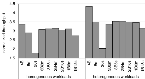
Figure 7. Average performance assuming a uniform thread count distribution and SMT in the homogeneous configurations.
