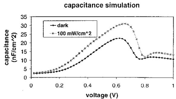
Fig. 4. SCAPS-1D simulation of the capacitance vs. voltage characteristics in the dark and under illumination (the same simulation parameters as for Figure 2 were used). The junction doping profile and the doping concentration in the vicinity of the back contact were deduced from the measurements.
