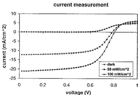
Fig. 1. Measured current vs. voltage of a CdS/CdTe cell from ANTEC for different illumination intensities (AM1.5G spectrum).
