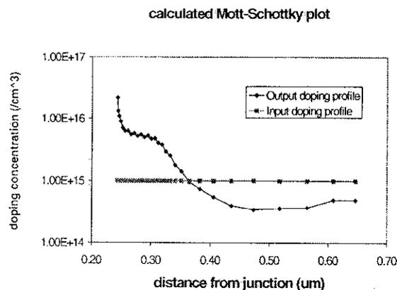
Fig. 6. CIS doping profile, deduced from the slope of the simulated  $1/C^2$  vs.  $V$  curves. The figure shows a spatially varying doping concentration. However, the absorber was assumed to be uniformly doped.
