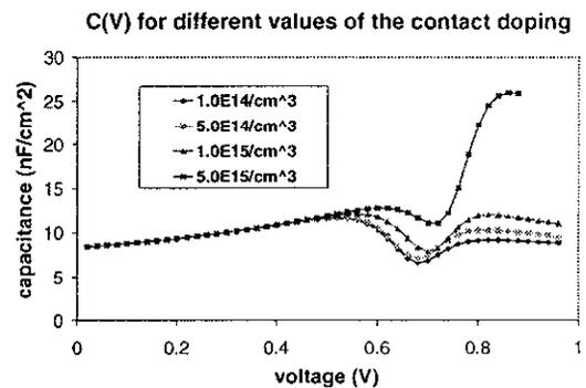
Fig. 5. SCAPS-1D simulation of the capacitance of a CdTe cell. For all curves, the junction doping equals  $10^{15}/\text{cm}^3$  and the Schottky barrier height 0.5 eV. The parameter is the doping concentration in the vicinity of the back contact.
