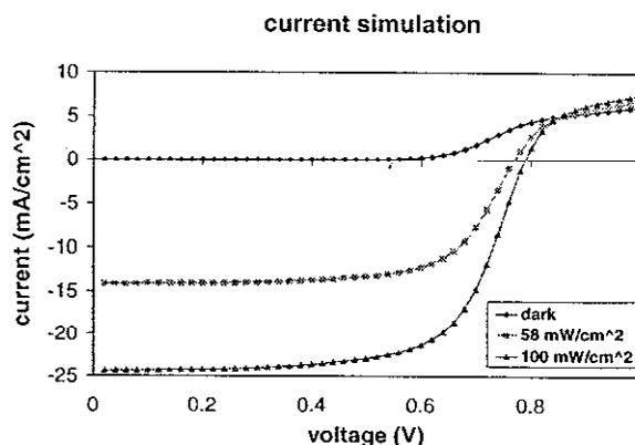
Fig. 2. SCAPS-1D simulation of the current voltage characteristics.
