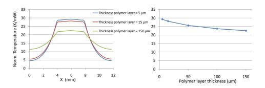
**Figure 8.28:** Normalized temperature distribution along the X-axis (left) and normalized VCSEL temperature (right) in function of the polymer thickness above the VCSEL.
