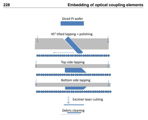
Figure 7.19: Schematic process flow for the fabrication of mirror plug components.
