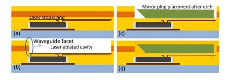
**Figure 7.28:** Schematic cross-sectional process flow for the embedding of mirror plugs into the layer build-up of the embedded optical link.
