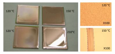
**Figure 6.13:** Pictures of 1  $\mu$ m thick sputtered Cu on a Truemode<sup>TM</sup> Backplane Polymer layer which was cured at 120°C, 150°C and 210°C.
