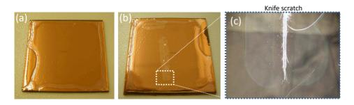
**Figure 6.16**: Scotch tape test (a) and scratch test (b)&(c) of a 30  $\mu$ m thick copper layer on top of a 1  $\mu$ m thin sputtered layer
