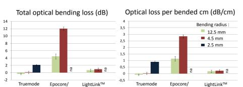
**Figure 4.24:** Total optical bending loss (left) according to the set-ups in Figure 4.23 and the recalculated losses per centimeter of bended waveguide length (right) for Truemode<sup>TM</sup> Backplane Polymer, Epocore / Epoclad and LightLink<sup>TM</sup> flexible waveguide foils.
