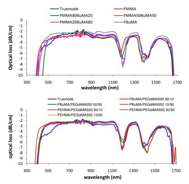
**Figure 2.8:** Optical bulk losses of Truemode<sup>™</sup> Backplane Polymer material and the different mixtures/materials.
