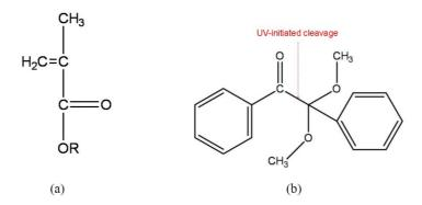
**Figure 2.3:** Basic structure of methacrylate (a) and of the photo-initiator Irgacure651 for the Truemode<sup>TM</sup> Backplane Polymer material.
