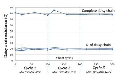
**Figure 8.20:** Evolution of the daisy chain resistance of an embedded IC on a rigid FR-4 board during temperature cycling.
