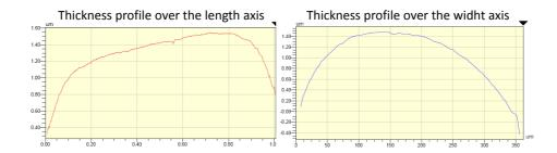
**Figure 5.13:** Thickness profile over the length and width axis of a polished 1 x 4 VCSEL array
