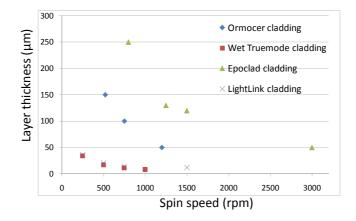
**Figure 3.4:** Layer thickness versus spin speed for 4 cladding materials on top of an FR4 substrate.
