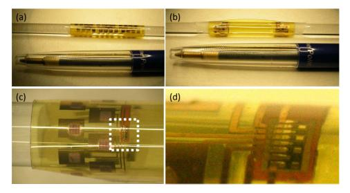
**Figure 8.15:** VCSEL and PD array package (inside one sample) rolled up around a cylinder with a 2 mm radius in both directions (a & b) and close-ups on the 1 x 4 VCSEL array (c & d).
