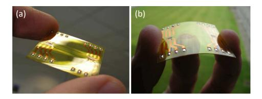
Figure 8.16: Finalized flexible active optical link substrate flat (a) and bended (b).
