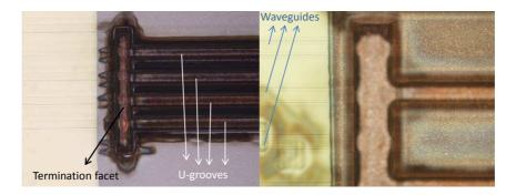
**Figure 7.34:** Laser ablated U-grooves for the embedding of optical fibers inside the optical foil.
