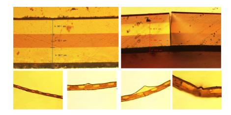
**Figure 4.14:** Truemode<sup>TM</sup> Backplane Polymer waveguide stack on top of a Polyimide foil and covered by a spincoated Polyimide layer (top left), breakage of the sample (top right) and delamination of the spincoated Polyimide layer (bottom).
