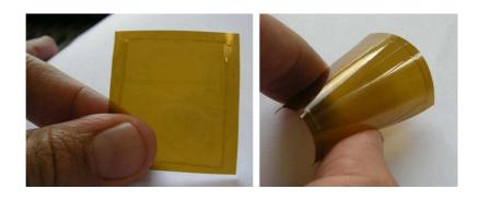
**Figure 4.8:** Laminated Truemode<sup>TM</sup> Backplane Polymer waveguide stack in between two Polyimide foils after lamination (left) and in bended state (right).
