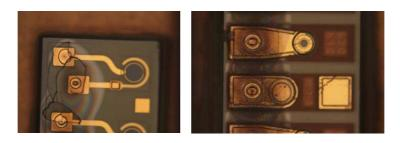
**Figure 6.22:** Pictures showing the local delamination around the laser ablated micro-via's, using PI2525 as an intermediate adhesion layer.
