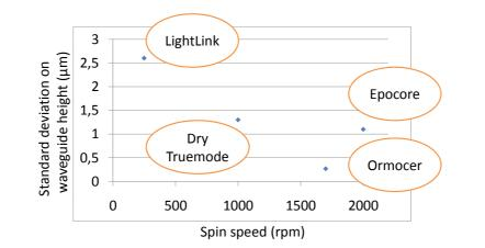
**Figure 3.15:** Spin speed versus waveguide height deviation for the 4 different materials, aiming at a waveguide thickness of  $40\mu m$ .
