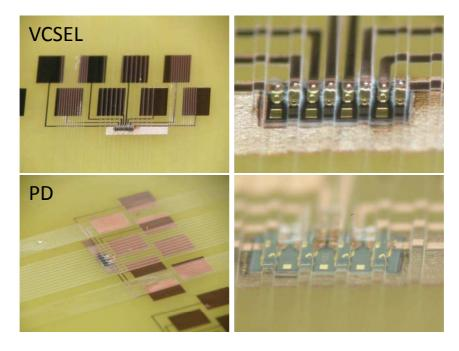
**Figure 6.6:** Microscope pictures of finished waveguides on top of an embedded VCSEL (top) and a photodiode (bottom).
