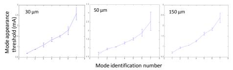
Figure 5.25: Mode appearance threshold per mode for a 150  $\mu m$  , 50  $\mu m$  and 30  $\mu m$  thick VCSEL
