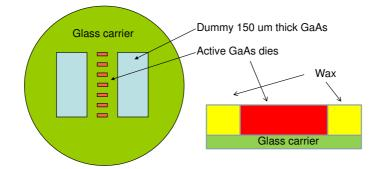
**Figure 5.7:** Wax mounting on glass carrier of 7 VCSEL arrays with 2 large (2 x 3 mm<sup>2</sup>) dummy dies (left) and cross-section (right)
