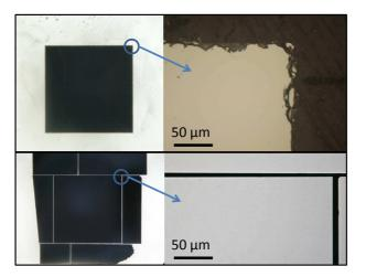
**Figure 5.18:** Edge damage after thinning of large GaAs dies (10 x 10 mm<sup>2</sup>) without the use of dummies (top) and with the use dummies (bottom).
