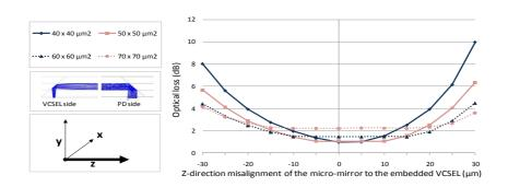
**Figure 7.10:** Optical loss simulation in function of the Z-misalignment of the micro-mirror with respect to the embedded VCSEL's for different waveguide dimensions.
