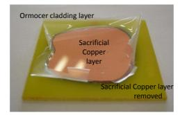
**Figure 4.3:** Partly released Ormocers<sup>®</sup> cladding layer processed on a copper coated FR4 board.
