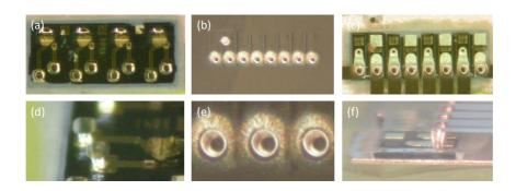
Figure 6.9: Photographs of  $CO_2$  laser ablated via's to embedded opto-electronic components
