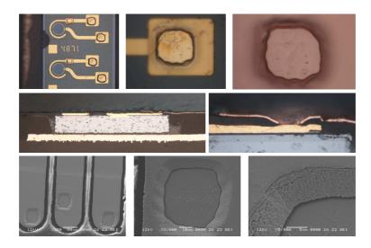
**Figure 6.19:** Microscopic pictures (top), cross-sections (center) and SEM pictures (bottom) of the contact pad delamination of Truemode<sup>TM</sup> Backplane Polymer.
