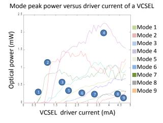
**Figure 5.24:** Power of each mode peak in the optical spectrum emitted by a multimode VCSEL versus the driver current.
