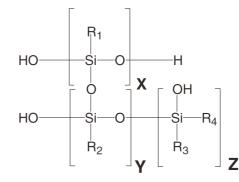
Figure 2.4: Inorganic / organic polymer backbone of LightLink<sup>TM</sup>.
