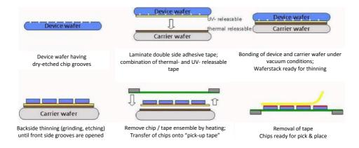
**Figure 5.4:** Schematic overview of the "dicing by thinning" principle followed by the transfer of the dies from the thinning carrier wafer to a low tac tape (pick &) place tape). (source:IZM)
