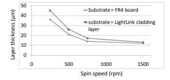
Figure 3.5: Influence of the underlying substrate on the spin speed curve of LightLink  $^{\rm TM}$  cladding material.
