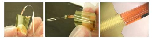
**Figure 7.36:** A completed optical waveguide foil connected to two optical fibers, bended in different directions (left and center) and a close-up of the fiber-connection (right).
