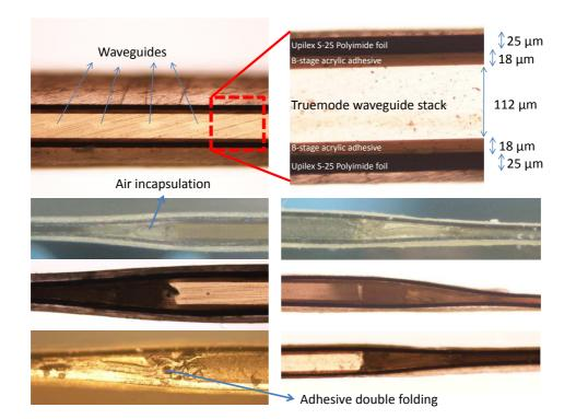
**Figure 4.7:** Cross-sections of a Truemode<sup>TM</sup> Backplane Polymer laminated waveguide stack with the layer thicknesses (top 2 pictures) and close-ups on the edges of the waveguide stacks (bottom 6 pictures)
