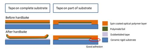
**Figure 4.9:** Edge adhesion approach for mounting of a Polyimide foil on top of a rigid substrate.
