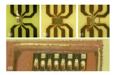
**Figure 7.29:** Picture of an embedded VCSEL with fan-out layer (a), of the laser stop island for the mirror plug cavity (b), of the cavity after wet etching of the cavity floor (c) and of a close-up on the waveguide facet (d).
