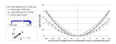
**Figure 7.3:** Optical loss simulation in function of the X-direction misalignment of the waveguides with respect to the active embedded VCSEL's and photodiodes.
