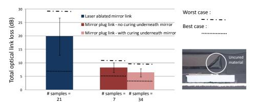
**Figure 8.4:** Average, standard deviation, worst case and best case of the total optical link loss for different coupling mirror situations.
