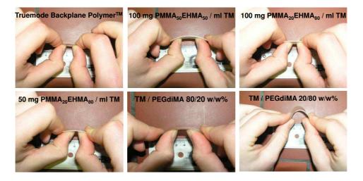
Figure 2.9: Visual comparison of the flexibility of the differnt developed mixtures materials.
