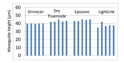
Figure 3.14: Waveguide height deviation for 5 samples of each material.
