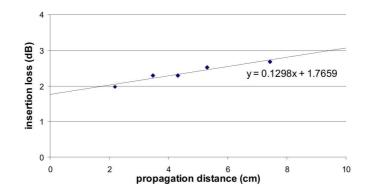
**Figure 4.20:** Cut-back optical waveguide propagation loss measurement for wet film Truemode<sup>TM</sup> Backplane Polymer laser ablated waveguides (Source: PhD-thesis Geert Van Steenberge)
