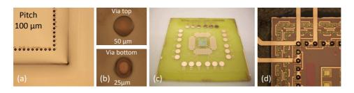
**Figure 6.27:** Pictures of the embedded IC (a) and the Excimer laser ablated micro-via's (b) after sputtering (a & b) and after etching (c & d ).
