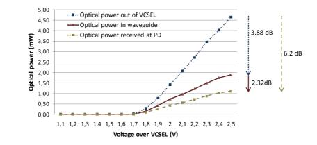
**Figure 8.6:** Results from the optical power loss measurement of both halfs of the embedded optical link.
