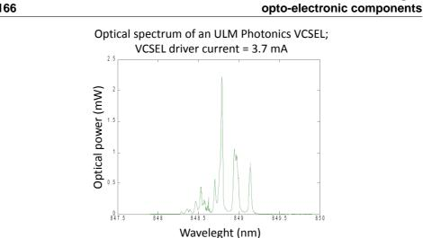
Figure 5.23: Optical spectrum of an unthinned ULM Photonics VCSEL, driven with a current of 3.7 mA.
