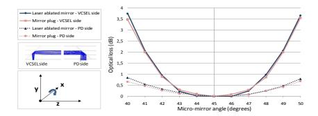
Figure 7.8: Optical loss simulation in function of the micro-mirror angle.
