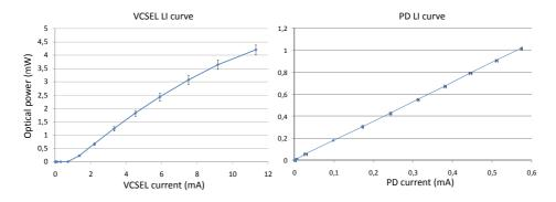
**Figure 8.1:** LI curve of an ULM Photonics 850 nm VCSEL ULM850-05-TT-C0104U (left) and a AlbisOptoelectronics photodiode PDCA04-70-GS (right).
