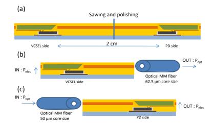
**Figure 8.5:** Set-up for the optical loss measurement of both halfs of the embedded optical link.
