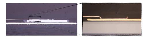
**Figure 6.20:** Cross-section of an Excimer laser ablated via through the SU-8 chip covering layer
