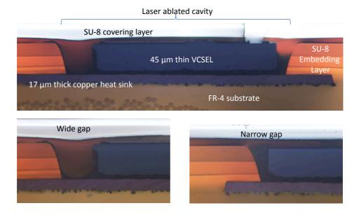
**Figure 6.5:** Cross-sectional photograph of a fully embedded 45  $\mu$ m thin VCSEL inside SU-8 material and a close-up on the filling of the VCSEL-cavity gap for a narrow and a wider gap.
