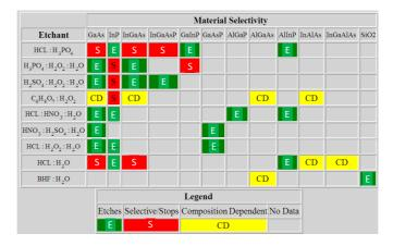
**Figure 5.3:** Material etch selectivity of the different etchant for the common compound semiconductor materials (Source: University of Maryland: Laboratory for Physical Sciences).
