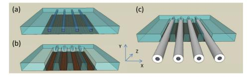
**Figure 7.32:** 3D schematic of the process flow to embed 125  $\mu$ m diameter optical fibers inside the optical waveguide foil.
