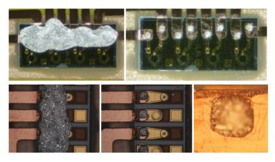
Figure 6.21: Metal paste via filling pictures.
