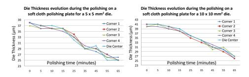
**Figure 5.9:** Chip thickness evolution during the polishing process for a 5 x 5 mm<sup>2</sup> and 10 x 10 mm<sup>2</sup> GaAs die
