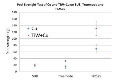
**Figure 6.14:** Peel strength test results of  $(1\mu m \text{ Cu})$ -strips and  $(50 \text{ nm TiW} + 1 \mu m \text{ Cu})$ -strips on top of a PI2525, SU-8 and Truemode<sup>TM</sup> Backplane Polymer layer.
