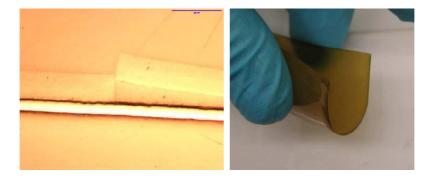
**Figure 4.12:** Cross-section of a fracture of a Truemode<sup>TM</sup> Backplane Polymer waveguide stack on top of a Polyimide foil (left) and a bended SU-8 layer stack on top of a Polyimide foil (right).
