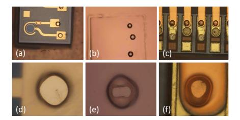
Figure 6.8: Pictures of Excimer laser ablated via's to embedded opto-electronic components
