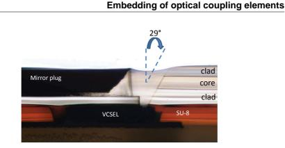
**Figure 7.13:** Cross-section of an embedded VCSEL array and mirror plug, showing the taper angle of the laser ablated mirror plug cavity side wall.
