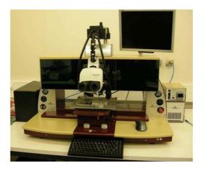
Figure 6.3: Dr. Treski fine-pitch placer installed in the cleanrooms of CMST Microsystems.
