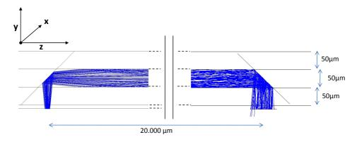
**Figure 7.2:** ZEMAX ray-tracing simulation set-up for the dimensional optical simulation of the embedded optical link.
