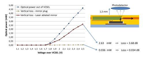
**Figure 8.3:** Optical power detected right above the VCSEL inside the optical link for laser ablated mirrors and mirror plug inserts.
