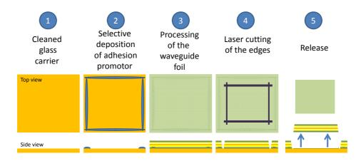
**Figure 4.15:** Schematic process flow of the release method for spincoated Polyimide on top of a float glass carrier, using selective adhesion promoter deposition.
