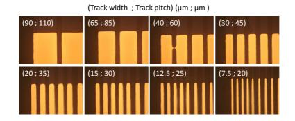
Figure 6.12: Copper fan-out etching resolution test
