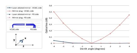
**Figure 7.6:** Optical loss simulation in function of the die tilt angle of the embedded VC-SEL/photodiode.
