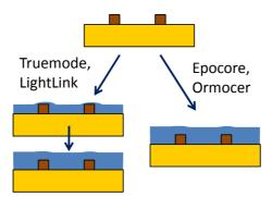
**Figure 3.20:** Applying of the uppercladding layer to cover the waveguides for Truemode<sup>TM</sup> Backplane Polymer , LightLink<sup>TM</sup> , Ormocers<sup>®</sup> and Epocore / Epoclad
