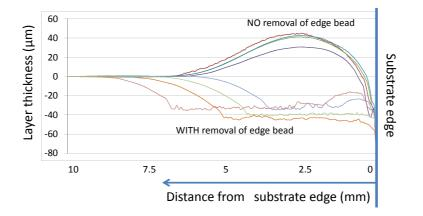
**Figure 3.2:** Edge layer thickness of wet film Truemode<sup>TM</sup> Backplane Polymer with and without edge bead removal (target layer thickness =  $40 \ \mu m$ )
