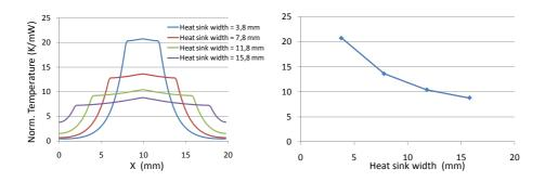
**Figure 8.25:** Normalized temperature distribution along the X-axis (left) and normalized VCSEL temperature (right) in function of the heat sink width.
