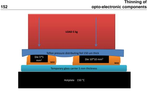
**Figure 5.8:** Wax mounting of 5 x 5 mm<sup>2</sup> and 10 x 10 mm<sup>2</sup> GaAs dies with the use of a Teflon pressure distribution foil for optimized leveling of the dies after mounting.
