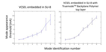
**Figure 8.34:** Mode appearance thresholds for embedded VCSEL's in SU-8 (left) and embedded VCSEL's in SU-8, with a 30  $\mu$ m Truemode<sup>TM</sup> Backplane Polymer layer spincoated and cured on top (right).
