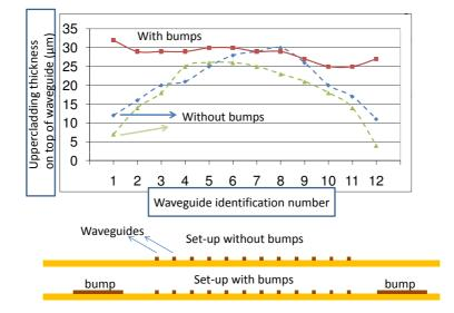
**Figure 3.21:** Schematic sketch of the bump principle for the reproducibility of the uppercladding thickness on top of the waveguides (bottom) and the uppercladding thickness for 12 different waveguides in a 1 x 12 waveguide array for bumped and non-bumped waveguide fabrication (top).
