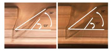
**Figure 7.16:** Cross-section of tilted laser ablation mirror trench, showing the different taper angle for the cladding and core material.
