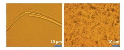
**Figure 4.11:** Microscopic picture of the surface of an untreated UPILEX S-25 Polyimide foil (left, the scratch is intentional to focus the microscope) and the same foil after sandblasting (right).
