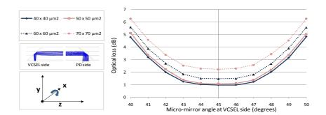
**Figure 7.12:** Optical loss simulation in function of micro-mirror facet angle for different waveguide dimensions.
