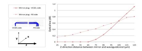
**Figure 7.7:** Optical loss simulation in function of the Z-distance between the micro-mirror and the start/end of the waveguide.
