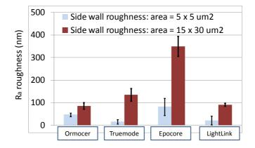
**Figure 3.18:** Ra roughness of waveguide side wall surfaces. Waveguides were fabricated in Ormocers<sup>®</sup>, Truemode<sup>TM</sup> Backplane Polymer, Epocore / Epoclad and LightLink<sup>TM</sup>. WYKO non-contact profilometer measurement on an area of 5 x 5  $\mu$ m<sup>2</sup> and on an area of 15 x 30  $\mu$ m<sup>2</sup>.
