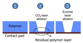
Figure 6.24: Schematic process flow for the opening of embedded contact pads.
