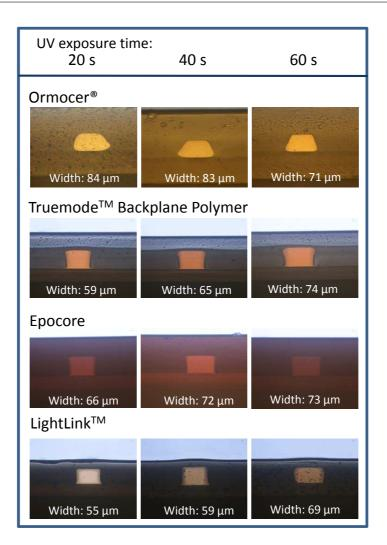
**Figure 3.11:** Cross-section of 250  $\mu m$  pitch waveguides in Ormocers® , Truemode<sup>TM</sup> Backplane Polymer , Epocore / Epoclad and LightLink<sup>TM</sup> material for different UV exposure times.
