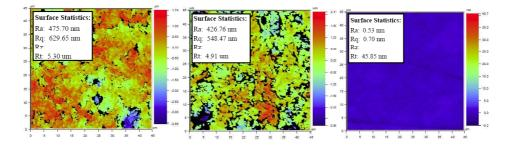
**Figure 5.17:** Non contact profilometer (WYKO) roughness measurements of a  $10 \times 10 \text{ mm}^2$  GaAs die on an area of  $50 \times 50 \mu \text{m}^2$ . Left: not thinned; center: after lapping ; right: after 65 minutes polishing
