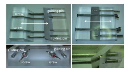
Figure 7.20: 45 degree mirror plug polishing tool.
