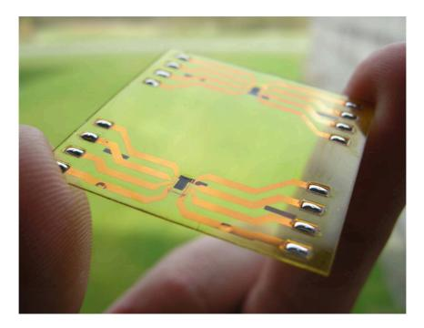
Figure 9.1: Picture of a 180  $\mu$ m thin foil with embedded VCSEL-to-PD links and galvanic interconnections.
