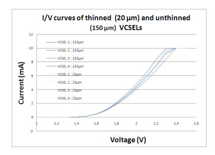
Figure 5.19: I/V Curves of 4 different VCSEL's in unthinned (150  $\mu m$  ) and in thinned (20  $\mu m$  ) status
