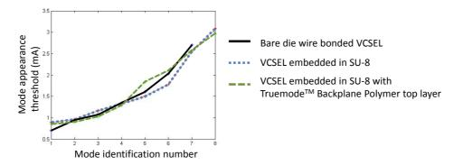
**Figure 8.35:** Comparison of the mode appearance thresholds for bare die wire bonded VCSEL's, embedded VCSEL's in SU-8 and embedded VCSEL's in SU-8, with a 30  $\mu$ m Truemode<sup>TM</sup> Backplane Polymer layer spincoated and cured on top.
