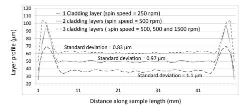
**Figure 3.7:** Planarization of a waved FR4 surface by spincoating LightLink<sup>™</sup> cladding
