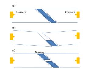
**Figure 7.21:** Dummy approach for the correct clamping of the mirror plug motherpiece in the PMMA 45 degree polishing tool.
