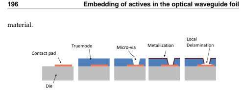
**Figure 6.18:** Schematic overview of the contact delamination problem during the embedding of actives inside Truemode<sup>TM</sup> Backplane Polymer material.
