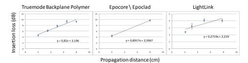
**Figure 4.19:** Cut-back optical waveguide propagation loss measurements for Truemode<sup>TM</sup> Backplane Polymer , Epocore / Epoclad and LightLink<sup>TM</sup> flexible waveguides.
