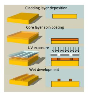
**Figure 3.9:** Schematic process flow for the fabrication of photolithographic optical waveguides.
