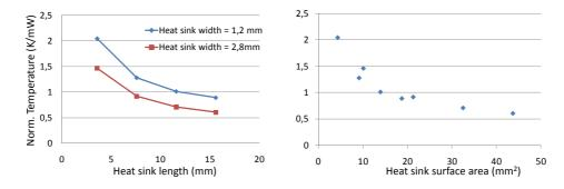
**Figure 8.32:** Normalized VCSEL temperature in function of the heat sink length for 2 different heat sink widths (left) and normalized VCSEL temperature in function of the heat sink total surface area (right).
