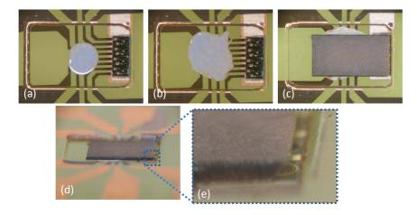
**Figure 7.30:** Pictures of the dispensing of the glue (a), the manual spreading of the glue (b), the placing of the mirror plug (c) and a close-up (d) & (e).
