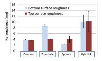
**Figure 3.17:** Ra roughness of waveguide top and bottom surfaces. Waveguides were fabricated in Ormocers<sup>®</sup>, Truemode<sup>TM</sup> Backplane Polymer, Epocore / Epoclad and LightLink<sup>TM</sup>. WYKO non-contact profilometer measurement on an area of 50 x 50  $\mu$ m <sup>2</sup>
