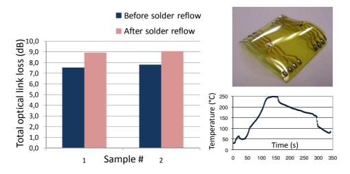
**Figure 8.23:** Total optical link loss changes and substrate deformation due to exposure to a standard solder reflow temperature cycle.
