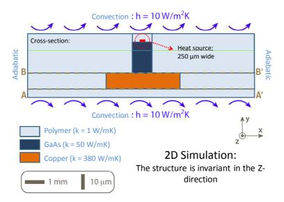
Figure 8.24: Two dimensional cross-sectional model overview.
