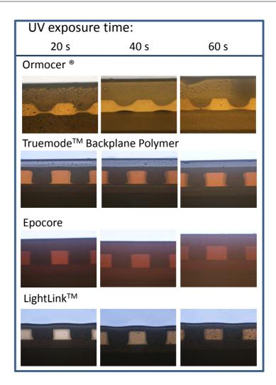
**Figure 3.12:** Cross-section of 125  $\mu$ m pitch waveguides in Ormocers® , Truemode<sup>TM</sup> Backplane Polymer , Epocore / Epoclad and LightLink<sup>TM</sup> material for different UV exposure times.
