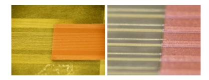
**Figure 7.33:** Copper island underneath the waveguides stack as laser stop for the U-grooves for optical fiber embedding.
