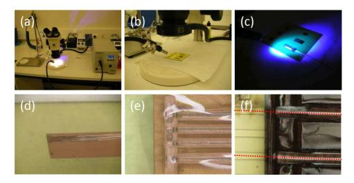
**Figure 7.35:** Mounting of the optical fibers inside the laser ablated U-grooves (a, b & c), side view of the mounted fibers (d) and top view (e & f).
