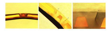
**Figure 4.13:** Damage of the optical layers at the waveguides due to a local peak in tensile stress in a Truemode<sup>TM</sup> Backplane Polymer waveguide stack on top of a Polyimide foil.
