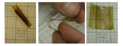
**Figure 4.10:** Examples of failure systems curling, cracking and delamination after processing of waveguide layers on top of an untreated Polyimide foil.
