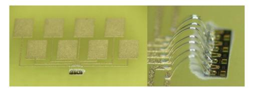
Figure 5.20: Wire bonded VCSEL package for optical characterization of a thinned VCSEL
