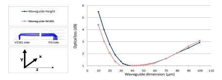
Figure 7.9: Optical loss simulation in function of the waveguide height and width.
