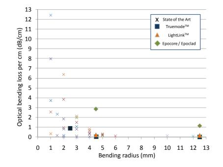
**Figure 4.25:** Bending losses of Truemode<sup>TM</sup> Backplane Polymer , LightLink<sup>TM</sup> and Epocore / Epoclad flexible waveguides versus the bending losses of state-of-the-art flexible waveguides.
