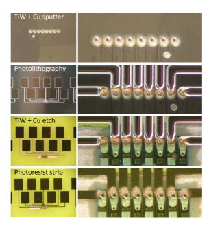
**Figure 6.11:** Process flow for the metallization of CO<sub>2</sub> laser ablated via's and fan-out from and to embedded opto-electronics in SU-8.
