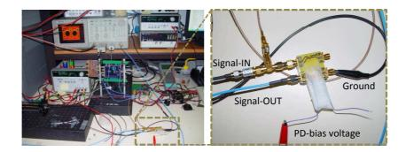
**Figure 8.13:** Set-up used to connect the optical link to a pattern generator to generate an eye diagram (left) and a close-up on the wired sample (right).
