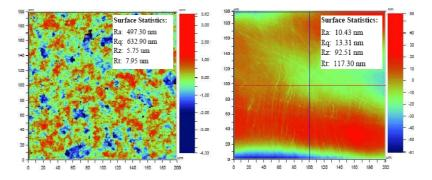
**Figure 5.14:** Backside roughness measurement with a non-contact profilometer (WYKO) of a lapped (left) and a polished (right) 1 x 4 VCSEL array
