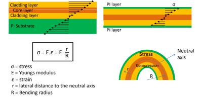
Figure 4.2: Principle of the neutral axis executed on the waveguide stack.
