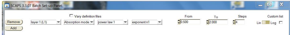
Fig. 9 Example of a batch parameter setting of an absorption model, The ‘power1’ model is set to be present (all other models remain present or absent as was set previously by the user interface or script). The model parameter n_1 will be varied over the values 0.5, 1.0, 1.5 and 2.0.
