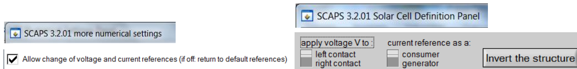
Figure 3.2 Setting user reference conventions for voltage and current. Left: checkbox in the More Numerical Settings Panel. Right: new facilities in the Solar Cell Definition Panel.
