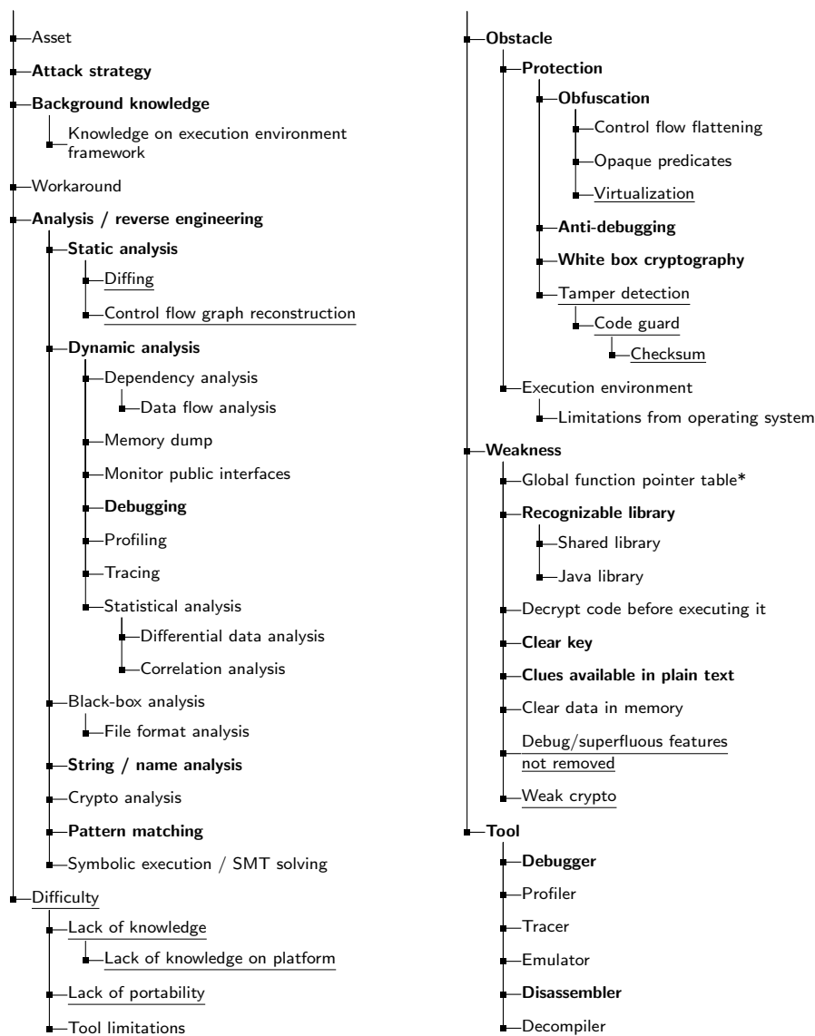
Fig. 3: Taxonomy of extracted concepts (part I): the analysis methods and tools hackers may use ( Analysis / reverse engineering , Tool ), weaknesses in design and coding of the application to protect that may help the hacker tasks ( Weakness ), the difficulty hackers may experience when trying to perform an attack task ( Difficulty ), the protections a defender can place to limit certain attack steps ( Obstacle ), and other high-level concepts that characterize the hacking scenarios ( Asset , Attack strategy , Background knowledge , Workaround ). * indicates multiple inheritance; new concepts added during the second qualitative experiment are underlined ; concepts emerged in both experiments are in boldface .
