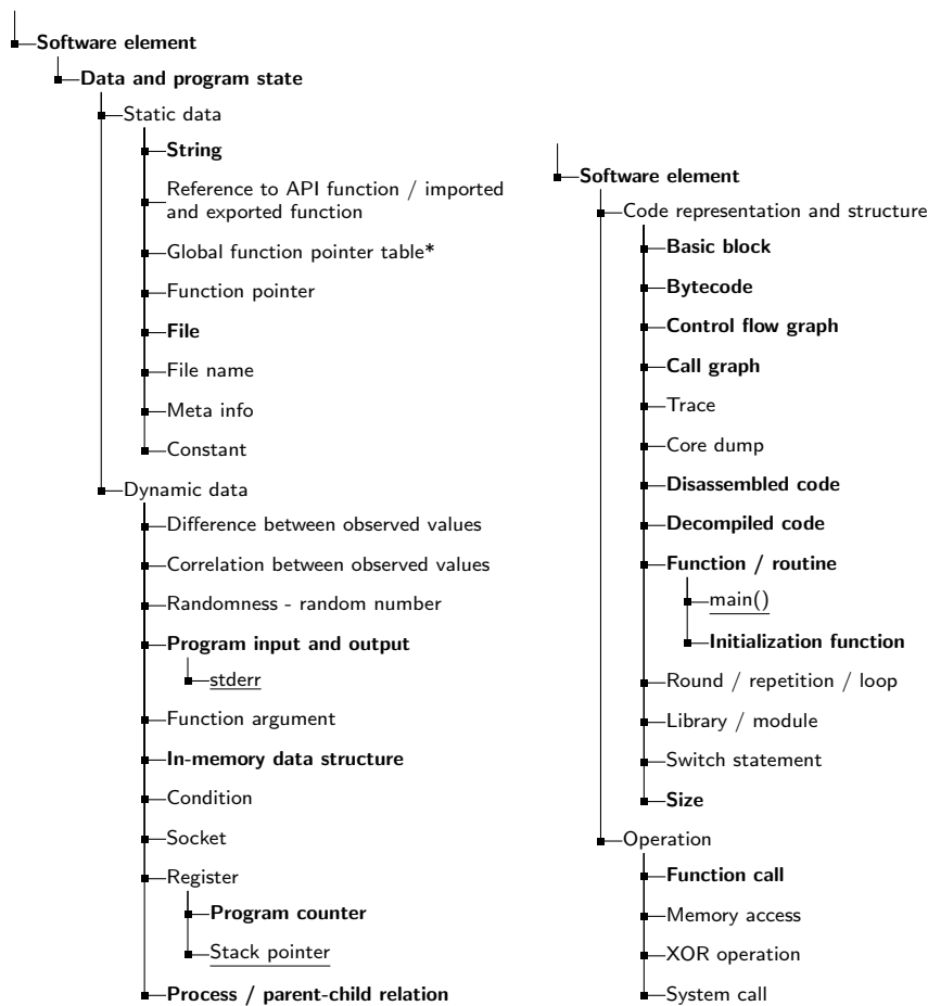
Fig. 5: Taxonomy of extracted concepts (part III): software elements. * indicates multiple inheritance; new concepts added during the second qualitative experiment are underlined ; concepts emerged in both experiments are in boldface .
