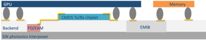
Fig. 5: Cross-section of the photonic-NoW GPU. GPU chips are connected to their local memory stack through electrical interposer interconnects; different GPU chips across the wafer are connected through waveguides in the wafer-scale photonic network.
